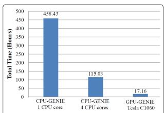
**Figure 4 GENIE execution time on the HDL study dataset.** GPU-GENIE achieves a speedup of 6.7 fold over CPU-GENIE using 4 Intel Xeon cores and 26.7 fold over CPU-GENIE using a single Intel Xeon core.
