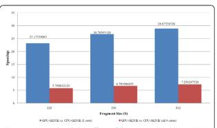
**Figure 5 A study of the effect of fragment size (S) on GPU-GENIE's speedup for the HDL study dataset.** Fragment size has an effect on the amount of speedup that is achieved by GPU-GENIE over CPU-GENIE. The largest speedup is attained for S = 512. As mentioned earlier, these experiments were carried out using a quad core Intel Xeon processor and an NVIDIA C1060 graphics card.
