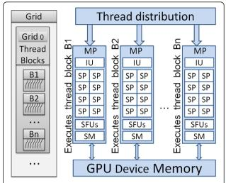
**Figure 1 NVIDIA GPU Architecture**. Simplified GPU Architecture: The grey rectangles of thread blocks are for illustration purposes and are not a physical part of the architecture. MP = Multi Processor, SM = Shared Memory, SFU = Special Functions Unit, IU = Instruction Unit, SP = Streaming processor (core).
