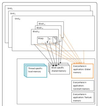
**Figure 2 CUDA Thread and Memory Hierarchy**. The dashed rectangle at the top half of the diagram shows the CUDA thread hierarchy while the large rectangle in the lower half shows the hierarchy of memory spaces in a CUDA device. To to T32 represent the threads contained in a warp. The current version of GENIE uses the global and local memory spaces that are represented by the orange and aqua colored boxes respectively.
