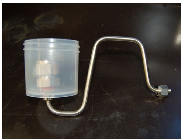
Fig. 2 Smooth bubble-burst nebulizer used for the preferential aerosolization process
