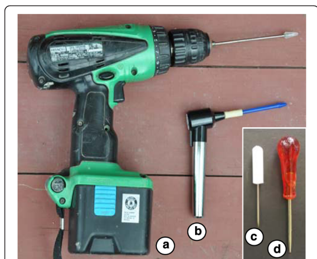
Figure 6 Grinding tools. a. Cordless drill (with rechargeable battery) with stainless steel pestle with Teflon end that fits inside a 1.5 ml microcentrifuge tube (purchased commercially). For hard tissues, a stainless steel rod without the Teflon end can be used for grinding. More force can be applied to the sample because of the smaller surface area. b. Battery-operated grinder with disposable pestle (purchased commercially). c. Manual grinder fashioned from a small screwdriver that has been ground so that the end fits into the bottom of a microfuge tube. d. Manual grinder fashioned from an awl that was ground to fit the bottom of microcentrifuge tube. The wider handle distributes the force on ones hand more evenly.
