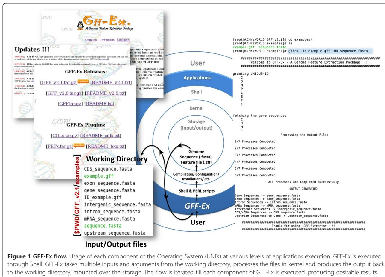
**Figure 1** GFF-Ex flow. Usage of each component of the Operating System (UNIX) at various levels of applications execution. GFF-Ex is executed through Shell. GFF-Ex takes multiple inputs and arguments from the working directory, processes the files in kernel and produces the output back to the working directory, mounted over the storage. The flow is iterated till each component of GFF-Ex is executed, producing desirable results.
