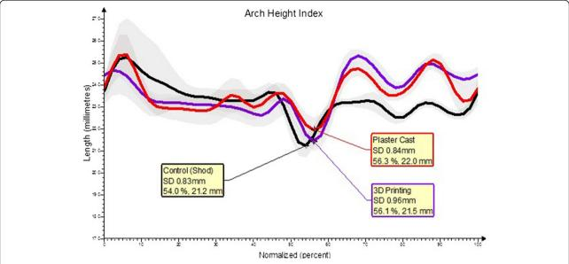
Figure 2 The Arch Height Index of the right foot measured using the Oxford Foot Model. Mean values, in millimeters (mm), from 30 gait cycles are illustrated for each trial, with (+/–) 1 standard deviation (SD) represented by the shaded area. Three conditions were compared: Control (shod), 3D Printing Orthotic and Plaster Casting Orthotic.
