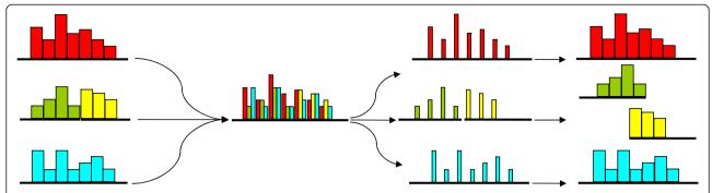
**Figure 1 Multiplex communication principle.** In communications technology and in other fields multiplexing is used to combine multiple independent packages of information into a continuous single signal that after transmission can be decomposed into the original information packages.
