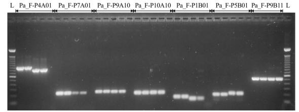
**Fig. 2** Amplification patterns of 7 SSR loci in *Passiflora edulis* (*first two lanes*, accessions 'IAPAR-06', 'IAPAR-123') and *P. alata* (*third and fourth lanes*, accessions '2(12)', 'SV3') following agarose gel (1.2%) electrophoresis at 3 V cm<sup>-1</sup> for 2 h. *Lane L*, 100 bp ladder
