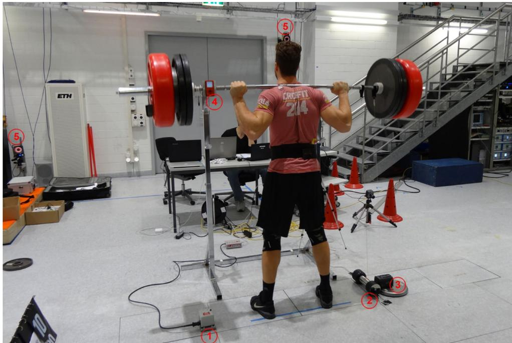
**Fig. 1** Simple measurement devices: 1 = T-force, 2 = Tendo unit, 3 = GymAware, 4 = Myotest, 5 = Vicon, the markers were placed at both ends of the bar
