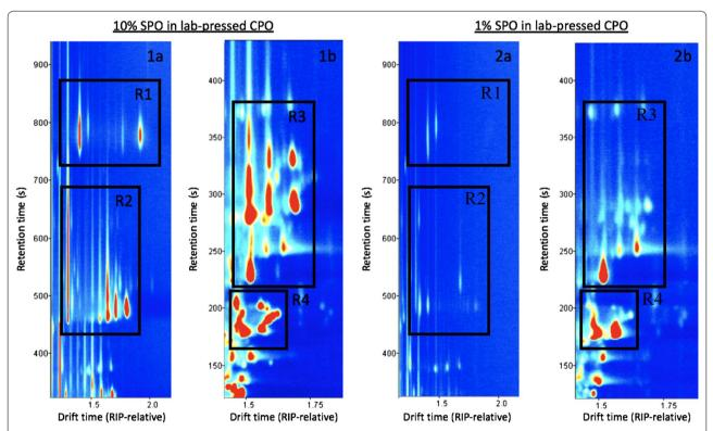
Fig. 1 A reporter view showing the proposed SPO markers. 1a shows region 1 and 2 in 10% SPO + lab-pressed CPO, whilst 1b shows regions 3 and 4. This format is replicated for 1% SPO + lab-pressed CPO in panels 2a and 2b
