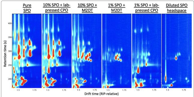
**Fig. 3** Reporter view showing region 4 of the SPO fingerprint across a range of samples. 10% SPO + lab-pressed CPO and 10% SPO + Mill 2 Dispatch Tank (M2DT) are most similar to the pure SPO fingerprint. 1% SPO + M2DT CPO and 1% SPO + lab-pressed CPO share similarities with both pure SPO and diluted SPO headspace. This trend is repeated for all regions of the SPO fingerprint across all spiked lab-pressed CPO and DT CPO (data not shown)
